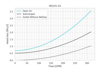
In the submerged case, opening pressure [mmH2O/inH2O] is the difference between the water level upstream and the water level downstream and in the open-air case to the inverted pipe.
